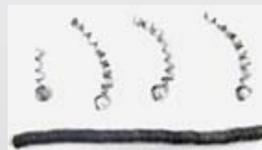
Chips by SM Chipbreaker (SUS304)
